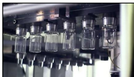
Use ISBM to manufacture bottles that have small to medium bodies and relatively small necks. We use ISBM to manufacture all of our Polyethylene Terephthalate (PET) bottles.
