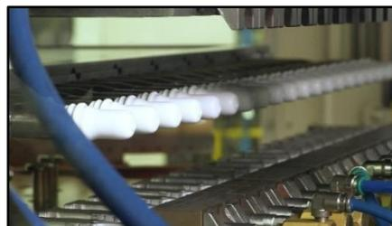
IBM is ideal for the production of HDPE, LDPE, and PP bottles that have small bodies and relatively small necks. We use IBM when manufacturing bottles with very tight neck tolerances.
